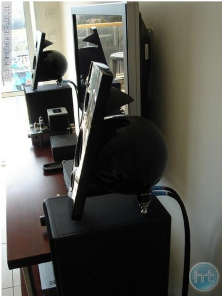
The sensitivity is 86db/1W/1M Terra LA, so it is likely that they will benefit if Oioztmdo dedicated amplifier. Amplifier is chosen mission distinguished the [Burson Audio PP-160](#) from the high - Australian End. Stereo amplifier that has a output of 85W and 160W in 8Ohms on 4Ohms these data to know to prepare for action the Terra LA easily.
